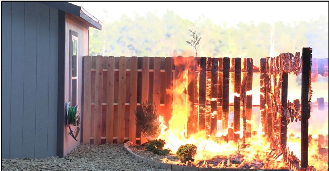
Figure 6.6. Fuels igniting between and around combustible back-to-back fencing.
