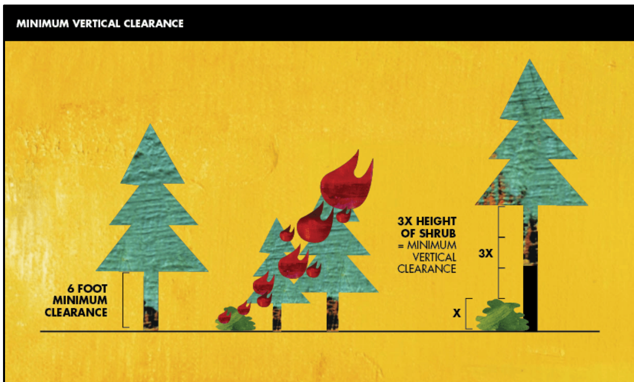
Figure D.4. Recommended minimal vertical clearance.
