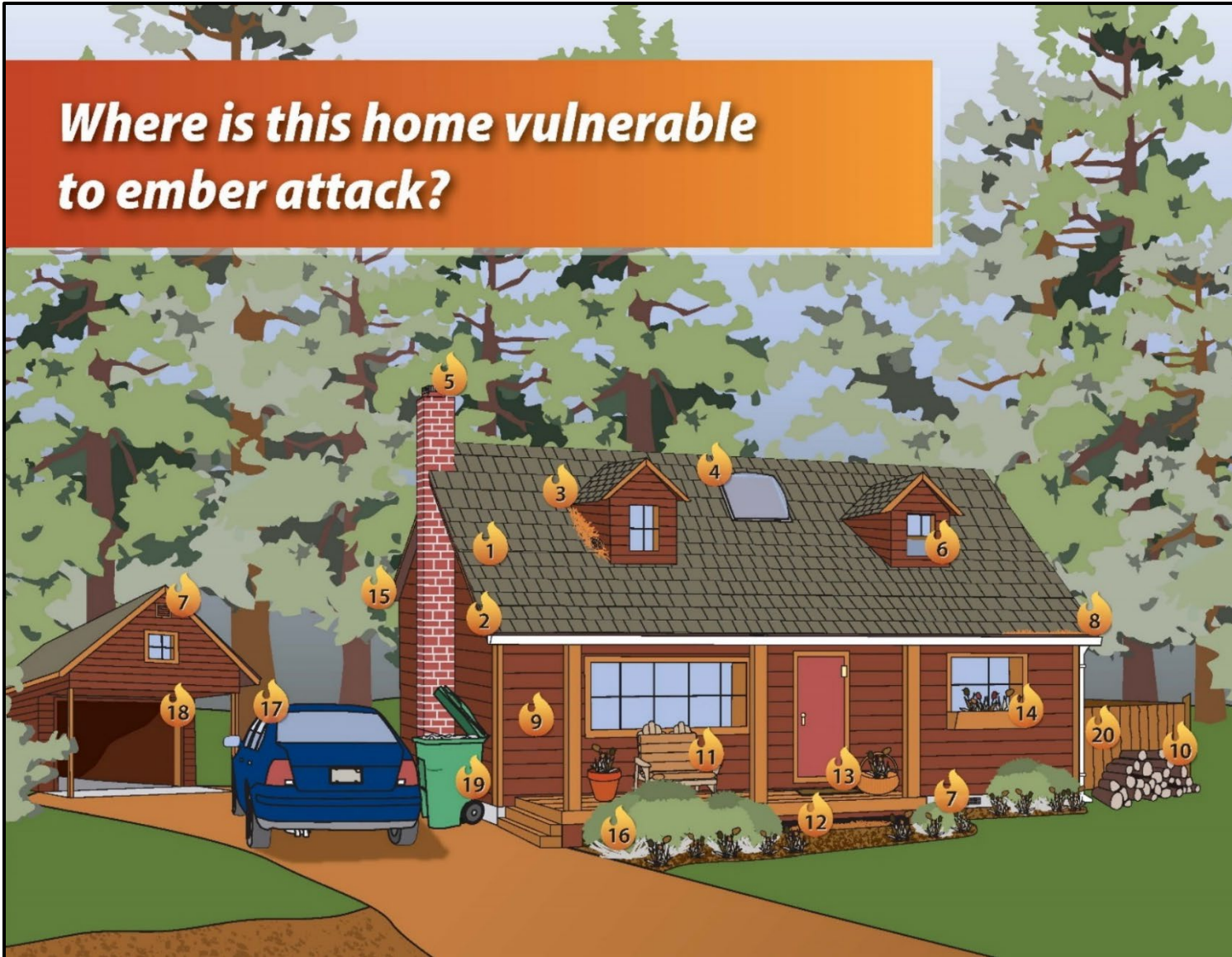
Figure 3.4. An example home in the WUI with ember ignition hazards identified by numbered flames.
