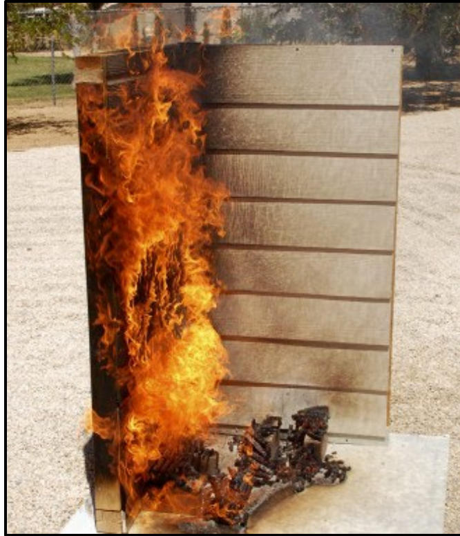
Figure 6.5. A two-sided wall showing a wood-composite siding material (left side) and a noncombustible fiber cement product (right side). A burning brand was used to ignite both sides; the right side made of noncombustible material did not incur significant damage from the flames.
