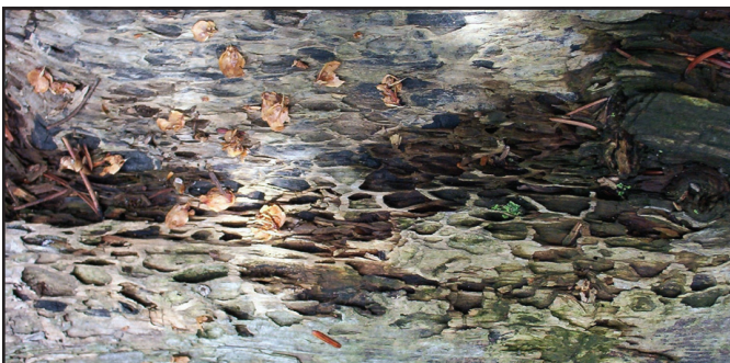
Figure 3. Spruce wood decayed by Phellopilus nigrolimitatus and subsequently weathered. Note the large, broad pockets separated by relatively undecayed wood.
