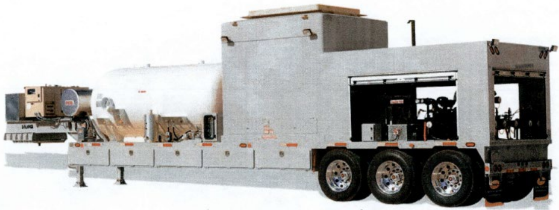
Hot oiler trailer to heat water on the fly.
