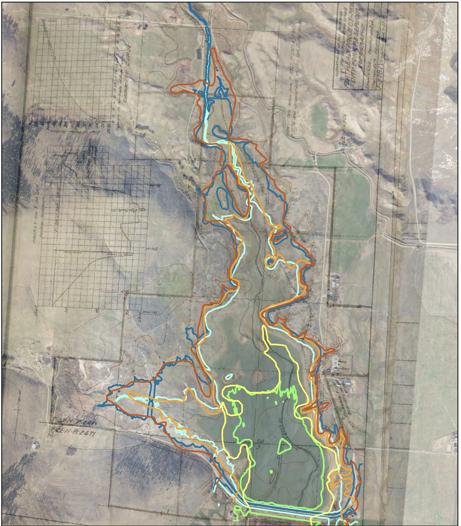
Figure 6: Lower Dry Fork Reservoir Original topobathymetric map over 2019 air photo base Comparison at 2840, 2850, 2855 foot contour intervals
