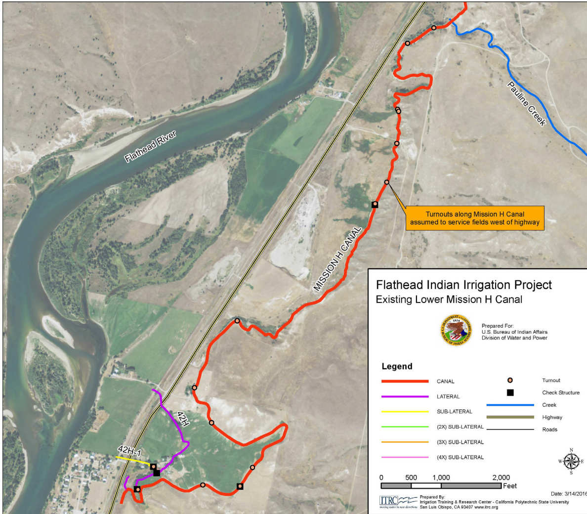
Figure 11. Existing conditions near the end of the Mission H Canal
