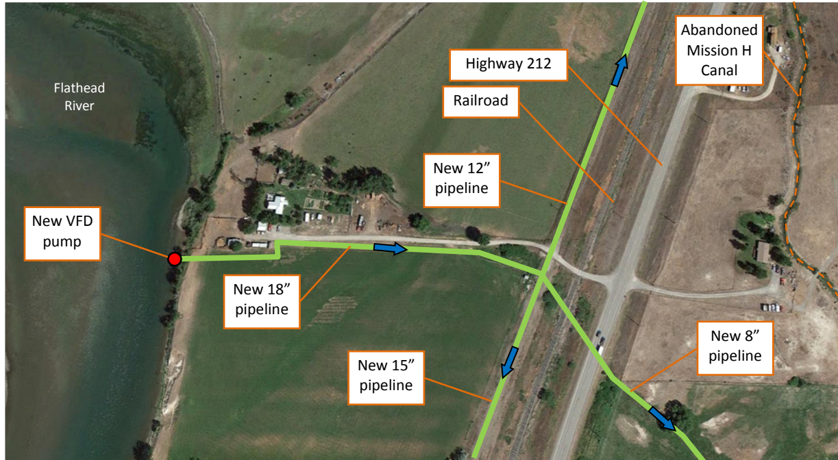
Figure 13. Approximate location for the new Lower Mission H Pump
