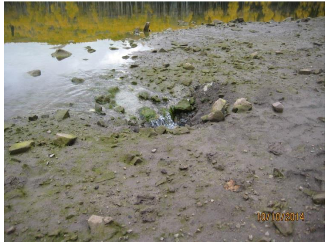
Figure 5. An Accessible Sinkhole in the Early Stages of Development – a Good Target for Plugging
