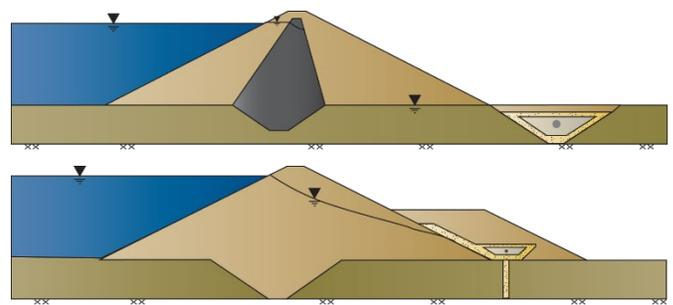
Figure 8: Potential Foundation Filter Configurations
