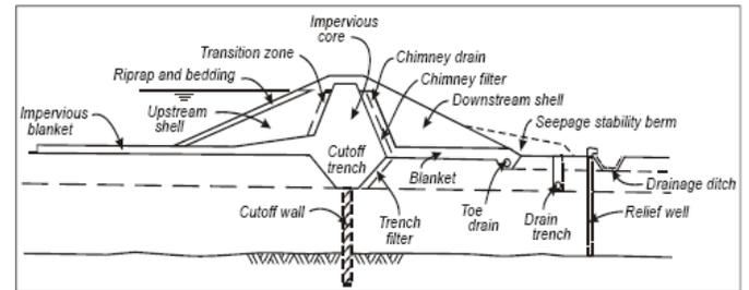
Figure 5: Potential Seepage and Internal Erosion Mitigation Features
