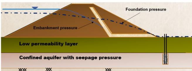
Figure 11: Relief Well Schematic
