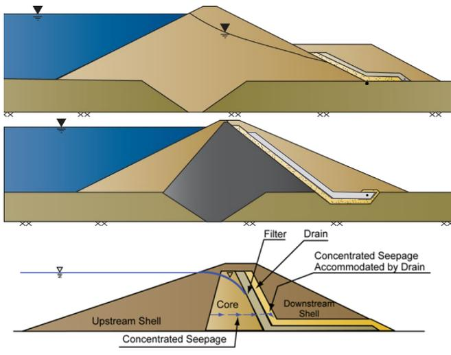
Figure 6: Potential Embankment Filter Configurations
