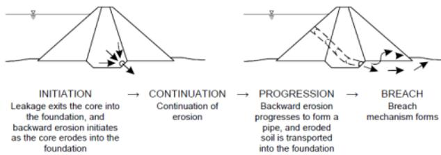
Figure 4: Internal Erosion of Embankment into Foundation PFM Nodes [3]
