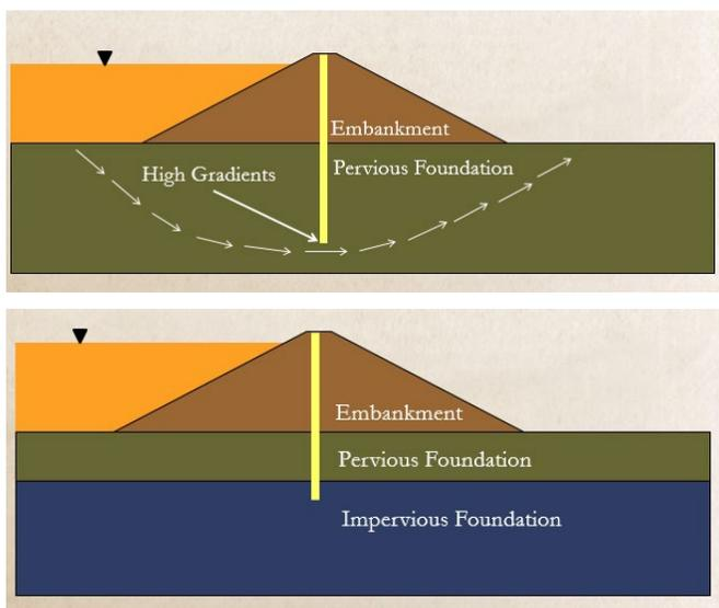
Figure 7: Potential Cutoff Wall Configuration
