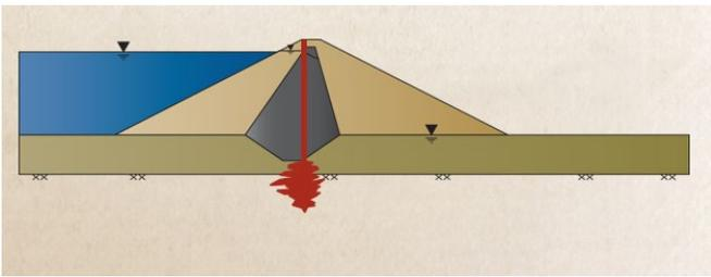
Figure 10: Foundation Grouting from the Dam Crest
