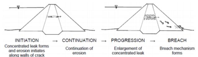
Figure 2: Internal Erosion through the Embankment PFM Nodes [3]
