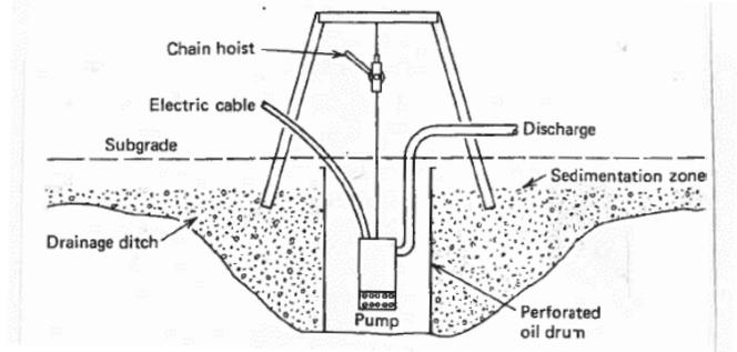
Figure 2 - Example of Simple Sump Installation [3]
