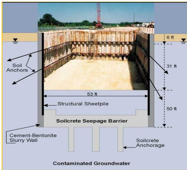
Figure 13 - A Jet Grout Bottom Seal Combined with a Barrier Wall (Courtesy of Hayward-Baker Inc.)
