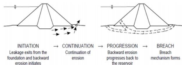
Figure 3: Internal Erosion through the Foundation PFM Nodes [3]
