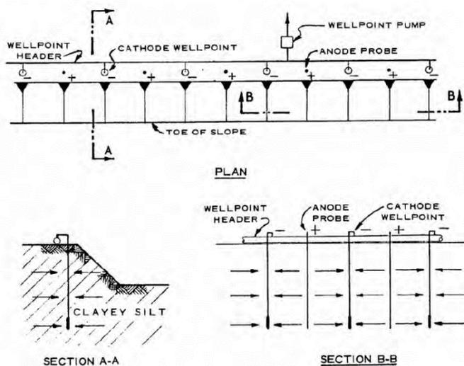
Figure 12 - An Electro-Osmosis Installation [5]
