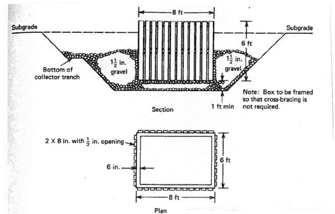
Figure 3: Example of More Complex Sump Installation [3]
