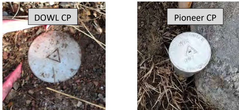
Figure 21 Typical Control Monuments Used
