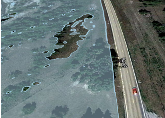
Figure 16 – 2D Calibration Results, Flooding on HWY 89, looking North
