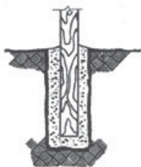
Post Backfilled with Concrete.
