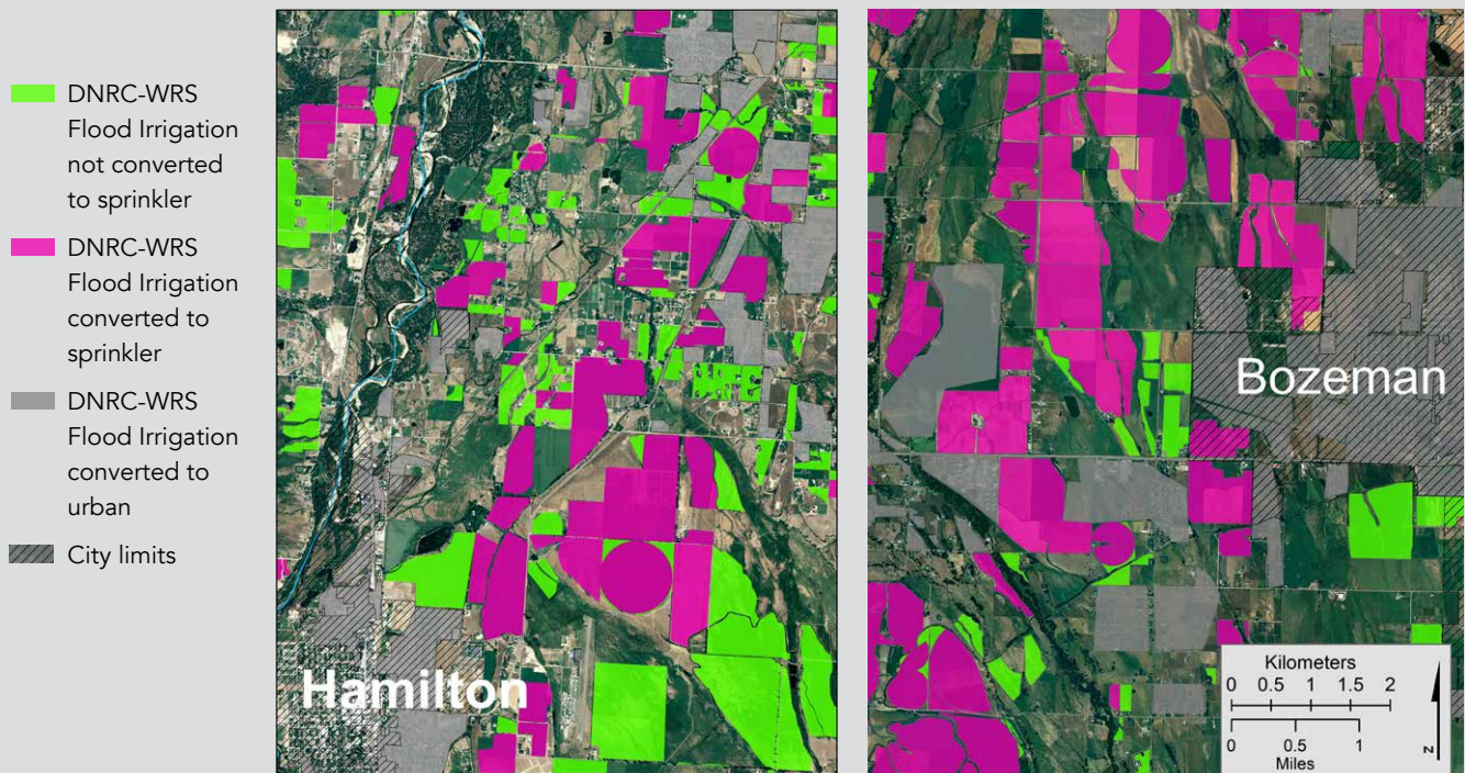
Figure 4 | Flood irrigated fields in Hamilton and Bozeman areas that were converted to sprinkler irrigation between the mid-20th century and 2019. Also shown are flood irrigated parcels not converted or converted to urban uses. Based on comparison of Montana Department of Natural Resources and Conservation Water Resources Surveys (1946-1971) and Montana Department of Revenue Final Land Unit Classification 2019. 54
