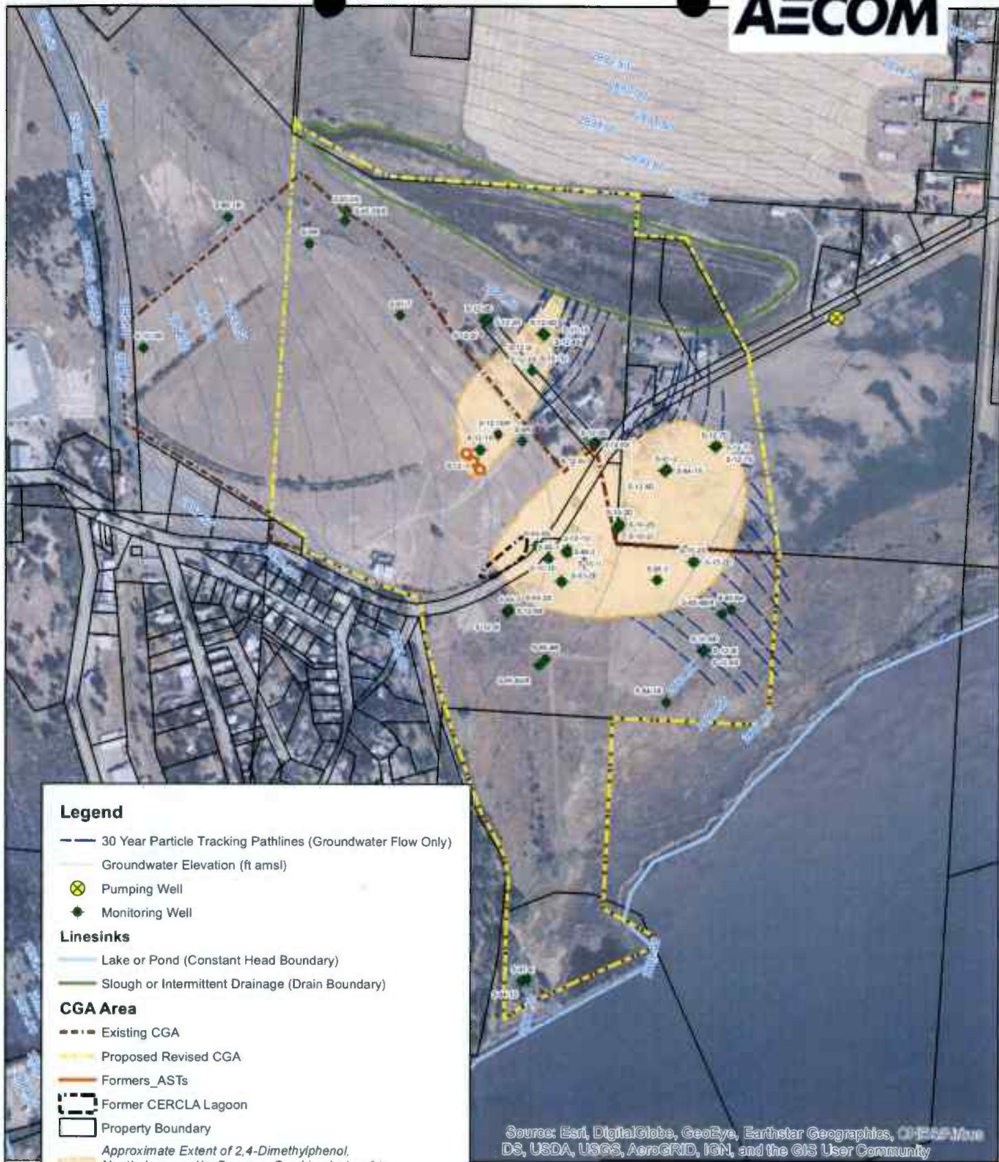
Figure 5 BNSF Site Somers, MT GFLOW Model Results Groundwater Elevation Pumping Well Rate 5 gpm
