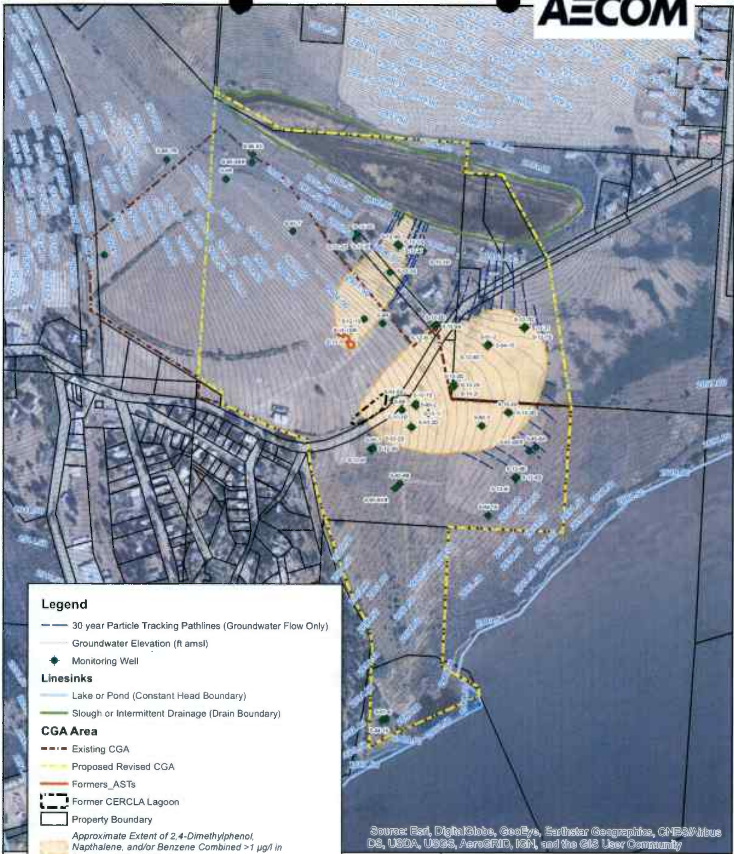
Figure 7 BNSF Site Somers, MT GFLOW Sensitivity Analysis Model Results Groundwater Elevation Alluvial Hydraulic Conductivity = 0.35 ft/d
