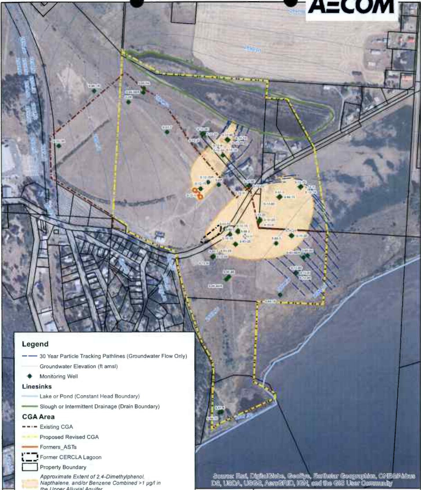
Figure 8 BNSF Site Somers, MT GFLOW Sensitivity Analysis Model Results Groundwater Elevation Alluvial Hydraulic Conductivity = 6.5 ft/d
